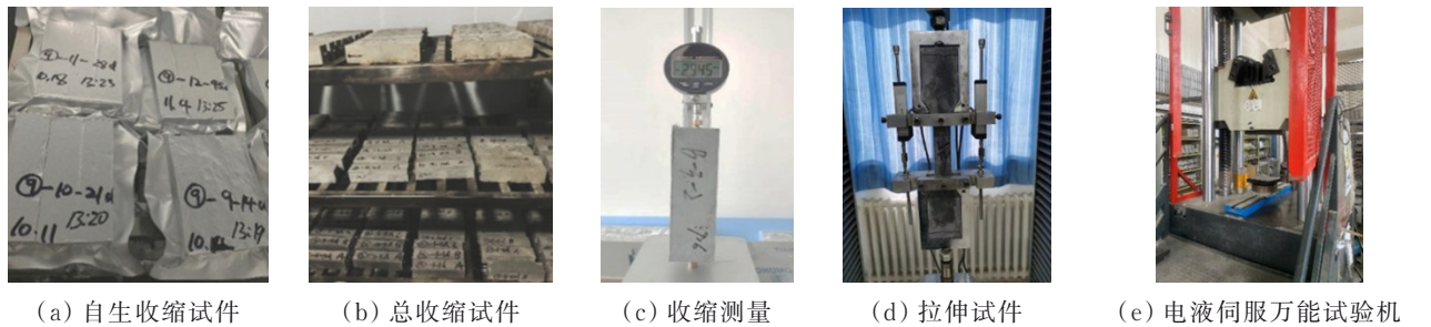
图 1 试件、试验仪器及设备 Fig.1 Specimen, test instruments and equipment
